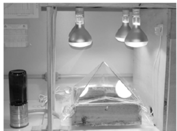
Fig.4. Experimental setup of solar still
